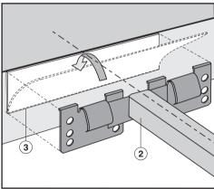
■ Position and attach the spring clips
