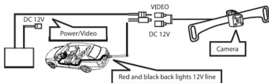
Complete all required connections so that all lines are hidden in vehicle.
