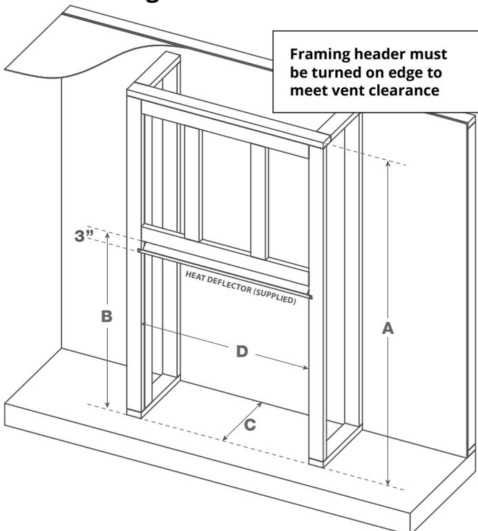
Combustible header can be reduced to 2" above unit if the fireplace chase is vented
