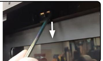
Figure 21.d Pull door latches
