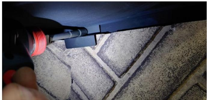
*Figure 20.b* Secure with the bracket using screw
