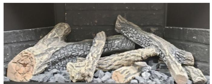
**Step 8:** Log **C** is placed between Log **B** and Log **H**, resting on Log **H**
