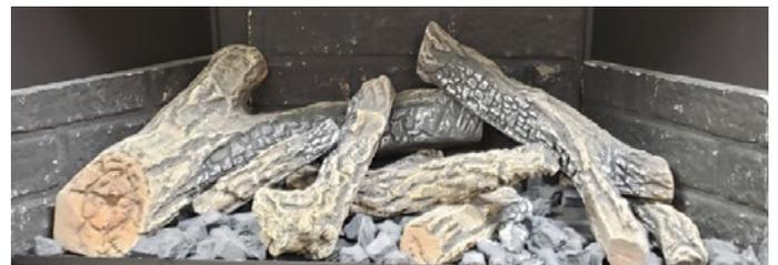
Only cover the burner with one layer of coals. Arrange the ember chips on top of the burner tray. DO NOT cover the pilot with logs.
