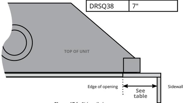
Figure 17.b Sidewall clearances
