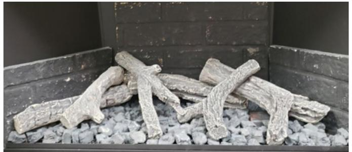
Only cover the burner with one layer of coals. Arrange the ember chips on top of the burner tray. DO NOT cover the pilot with logs.
