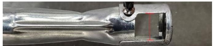
Depending on desired flame appearance recommended primary air adjustment limits: NG ⅛" – ¼" and propane ⅜" – Full open.
