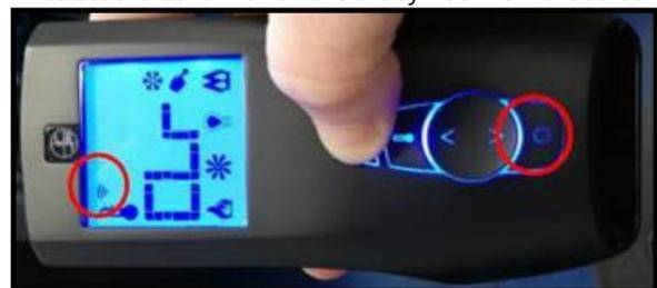
6. Release the Power On/Off button. The functionality is now enabled. The Tx Remote Command is now ready to be used.
