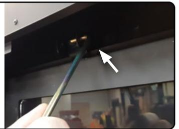
Figure 21.d Pull door latches
