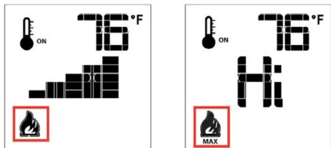
Figure 27.h Flame Level 5 and Flame Level Maximum
