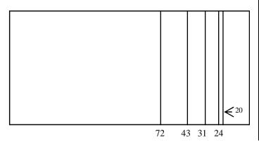
We use the same method to figure how far the top front center of the speaker's grille frame should be from the side walls. We take the width of the room, (14 feet) convert it from feet to inches, (14 x 12 = 168) and divide the result by odd numbers.
