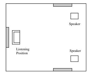
If your listening position is close to the wall behind you, mount some sound absorbent material, such as a hanging tapestry, directly behind your head. As with the diffusers for the side walls, experiment with a pillow or a folded natural-fiber blanket to verify the results before you acquire or mount the material.
