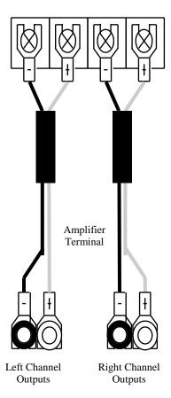
Bare wires should never come into contact with the aluminum dress plate while the amplifier is on. Amplifier damage could result.
