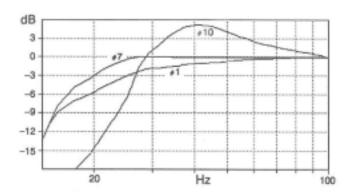
Once the room compensation controls have been set by a qualified technician, our experience is that the bass in most rooms sounds the most linear on high-quality music recordings with the Low-Frequency Contour set in the # 5 to # 8 range. Contour should always be the same for both speakers. Please remember that every room and system are different and that the nominal position in your system may be higher or lower due to room characteristics or personal preferences.
