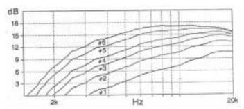
After you decide which contour setting provides the best high-frequency characteristics for your room, use the High-Frequency Level control to adjust the rear tweeter level. Each higher number increases the output of the rear tweeter by about 11/2dB.
