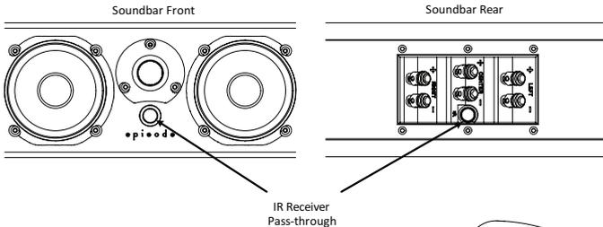
To maintain accurate IR reception, a spacer has been included to allow for the front edge of the IR receiver to be flush with the back of the grille cloth. This will ensure that IR reception is at its maximum level.
