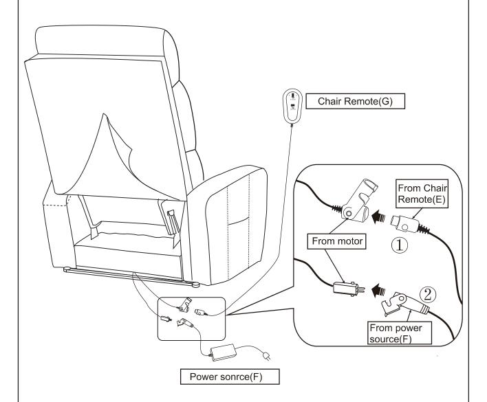
No.1 wire connect the motor and the wire from Chair Remote(D), No.2 wire connect the motor and power source (C).
