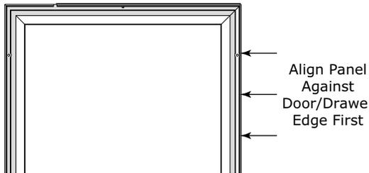
**Due to differences in floor construction or surrounding cabinetry, the panel may not sit flush with the top of the door/drawer.**
