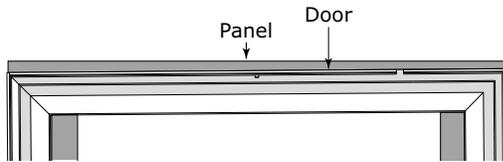
9. Secure integrated panel to door/drawer using clamps. A robust tape may also be used. U-Line recommends the use of bar clamps to secure the panel to the door/drawer. If using tape, be certain the tape will not damage panel finish upon removal.
