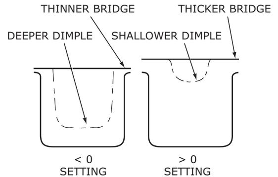
Ice thickness adjustments are made using the control panel as follows:
