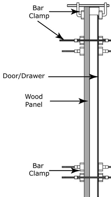
10. Using a 7/64" (3 mm) drill bit, drill 6 pilot holes into the wood panel 1/2" (12 mm) deep using the holes in the door/drawer frame as a guide.
