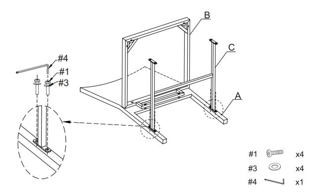
Step 3. Attach left front leg (part D) and right front leg (part E) to assembled unit (parts A, B & C) using bolts (part #1), flat washers (part #3) and allen wrench (part #4).
