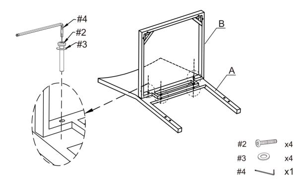
Step 2. Attach stretcher (part C) to back panel (part A) using bolts (part #1), flat washers (part #3) and allen wrench (part #4).
