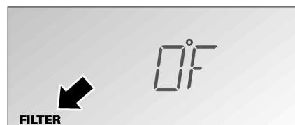
The age of the filter is close to the maximum life time. Order a new "UltraClarity" water filter.
