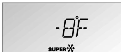
The **SUPER** symbol and the Fast freezing temperature are displayed.
