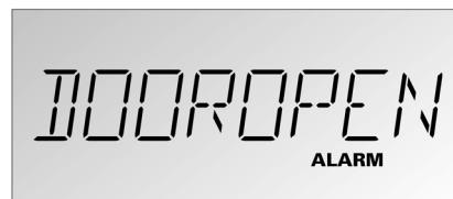
Close the door to switch off the warning signal.
