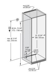
This is a fully integrated refrigerator-freezer appliance designed to be completely enclosed in a dedicated kitchen cabinet. This dedicated cabinet box must be constructed in accordance with the specified dimensions and must allow for sufficient air circulation to ensure proper operation. For more details about ventilation requirements, please refer to the Design Guide.
