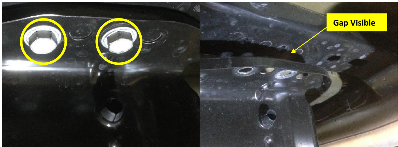
Figure 9 - JK-201 to Evap Canister Install
