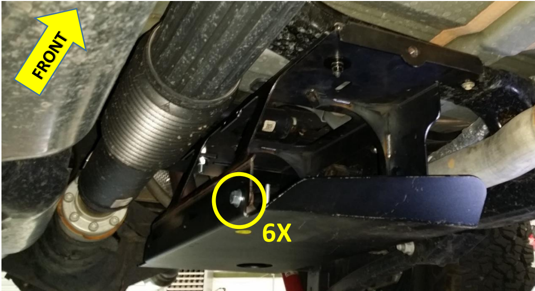
Figure 21 - JK-101 Mounted to Tank Bracket (Air Tank not shown)
