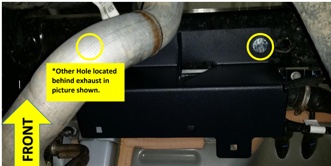
Figure 13 - JL-204 Adapter Bracket Bolted in Place
