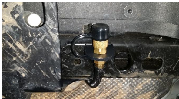
Figure 22 - Air Coupler Mounted To Bumper
