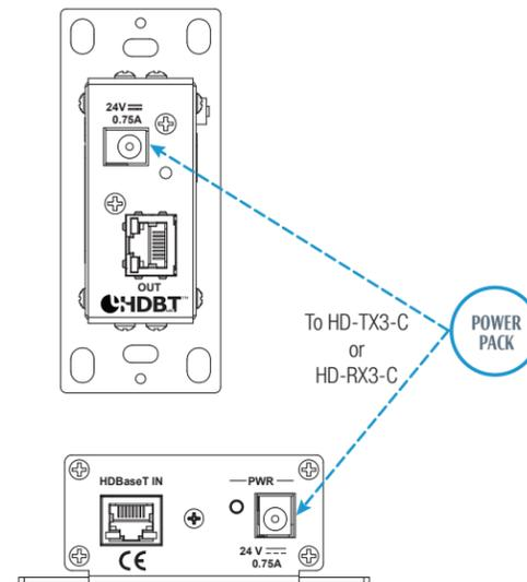
**NOTE:** The HD-TX3-C and HD-RX3-C are not HDBaseT PoE compatible; that is, the devices cannot be powered by—or supply power to—another HDBaseT device.
