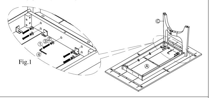
STEP 2: Attach the second Leg Frame (C) to Table Top (A), use the provided hardware as show on (Fig.2). Do not fully tighten, keep the assembly loose.
