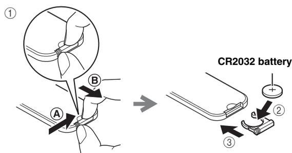
While pushing the release tab in direction (A), slide out the battery holder in direction (B).
