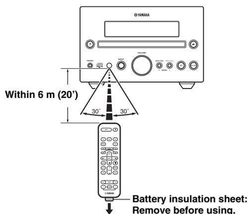
Use the remote control within 6 m (20') of this unit and point it toward the remote control sensor.
