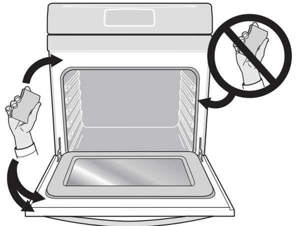
**Figure 6: Clean around the oven door gasket**
