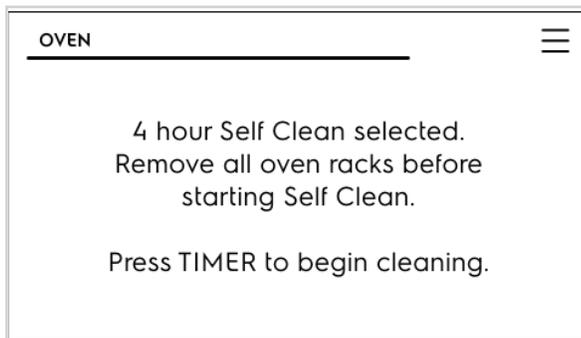
When the oven is set to run a self-clean cycle, the motor door lock will begin locking the oven door. Do not open the oven door while the lock motor is running or when any locking indicators or displays are showing. The oven door is completely locked in about 15 seconds. Once the oven door has locked, CLEAN will appear in the display indicating self clean has started.
