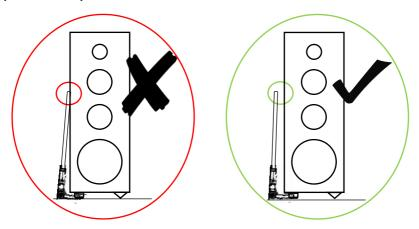
• While stabilizing the speaker, slowly raise the handle to lower the side of the speaker all the way to the ground.
