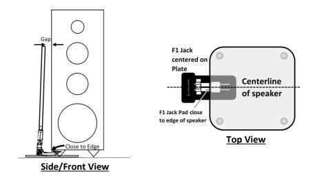
Position the F1 Jack underneath the speaker, centered on top of the floor plate. The speaker may need to be tilted in order to create enough space to slide the F1 Jack underneath it.
