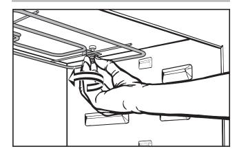
■ Uncrew the nut and lower the Browning/Broiling element.
