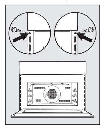
■ Open the door and use the screws supplied to secure the oven to the side walls of the cabinetry through the holes in the oven trim.
