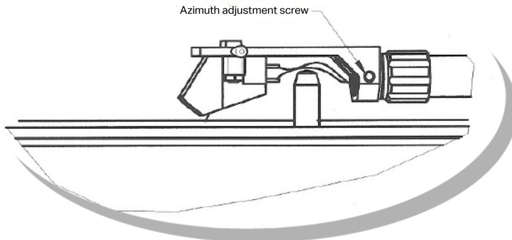
If cartridge body is declined to left or right side, please loosen Azimuth screw and turn headshell carefully in the opposite direction. The correct position is found, when the cartridge body is 100 parallel to the mirror (record). After setting has been finished, tighten Azimuth screw and start playback!
