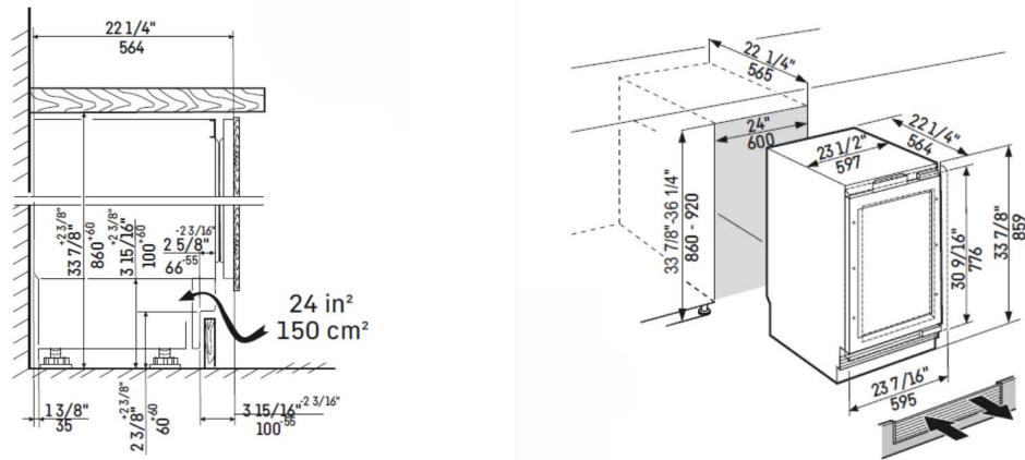
This is a built-in undercounter model which means that it is enclosed by a kitchen cabinet. This type of cabinet must be carefully constructed using the correct dimensions and it must provide suitable ventilation to ensure proper appliance operation.
