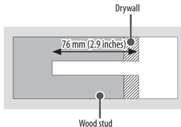
Use the Ø 4 mm drill bit for wood to drill holes with the depth of 76 mm (2.9 Inches). (Clean the drilled hole.)
