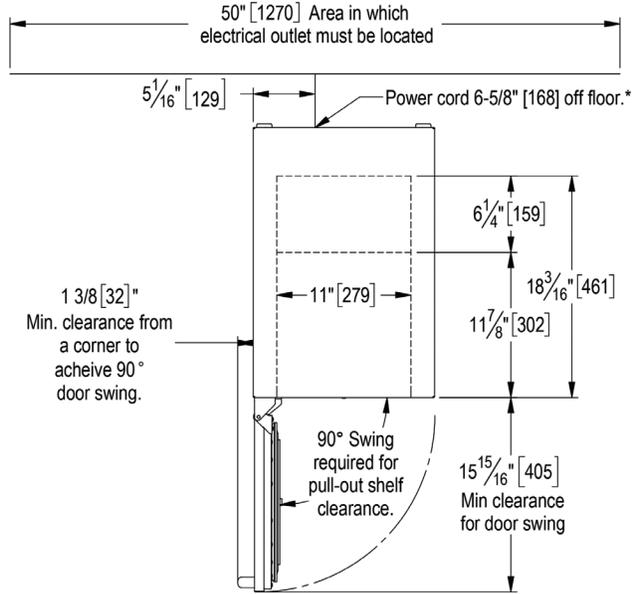
\* - Leg leveler can add 3/4" [19] to these dimensions when fully extended.
