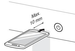
**3** Press and hold the **Temp.** button for 3 seconds or longer while continuing to hold your phone to the **Power** button.
