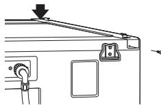
**3** Place the appliance on top of the washer, fitting the dryer feet into the side brackets as illustrated. Avoid finger injuries; do not allow fingers to be pinched between the washer and the appliance. Slowly slide the appliance toward the back of the washer until the side bracket stoppers catch the dryer feet.
