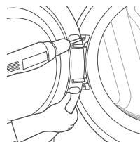
**4** Install the 2 decorative screws, the latch, and 2 latch screws removed in step 1 on the opposite side from which they were removed.
