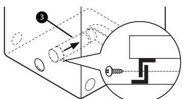
**3** Insert the 4" (10.2 cm) elbow **4** through the rear opening and press it onto the adapter duct. Be sure that the male end of the elbow faces down through the hole in the bottom of the dryer. Secure it in place with duct tape. Attach the cover plate **5** to the back of the dryer with the included screw.
