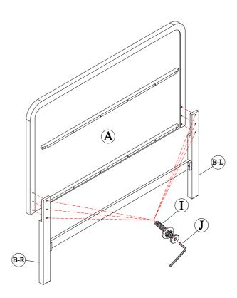
Attach Headboard Leg (L&R) (B) to Headboard (A) by using Bolt (I) and tighten with Allen Key (J).
