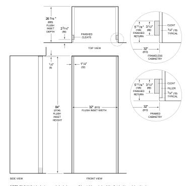
NOTE:31/2" (89) finished returns and shaded areas will be visible and should be finished to match cabinetry Shaded line represents profile of unit twit/1s" (19) panel.
