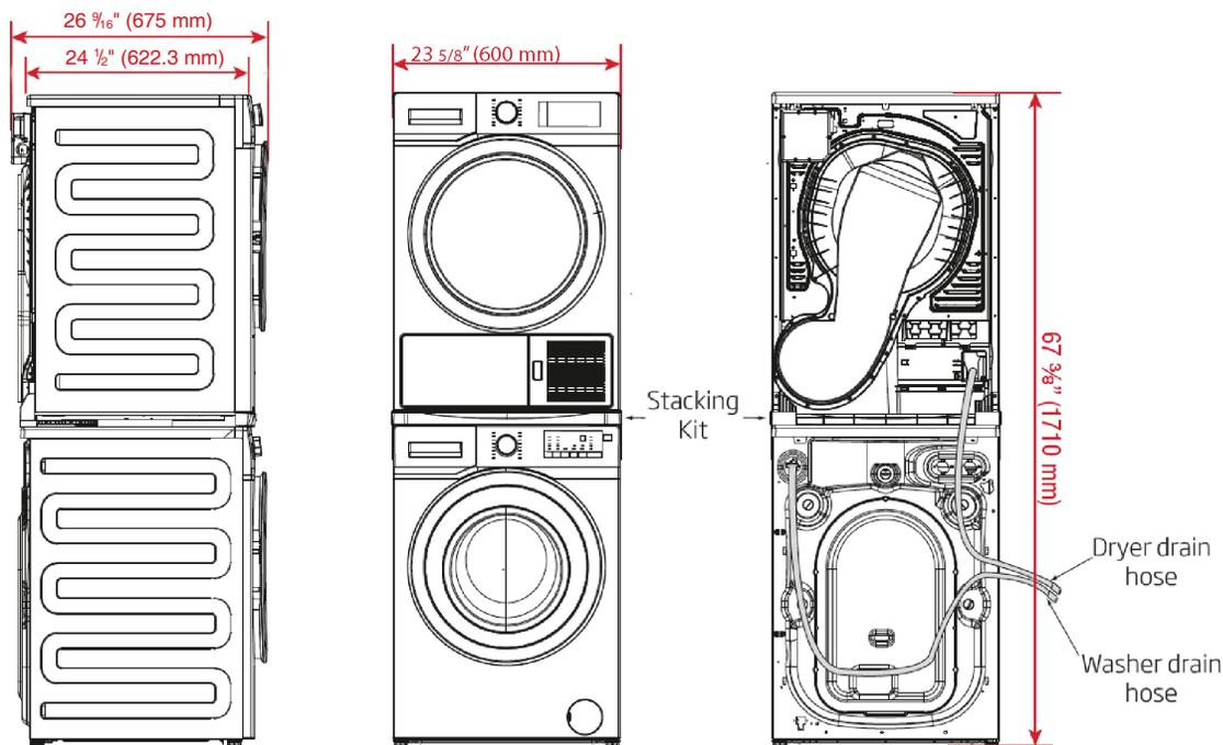
Stacked installation minimum air gap clearances:  $6 \frac{1}{4}''$  top,  $\frac{1}{2}''$  sides,  $\frac{1}{2}''$  back, front  $\frac{1}{2}''$
