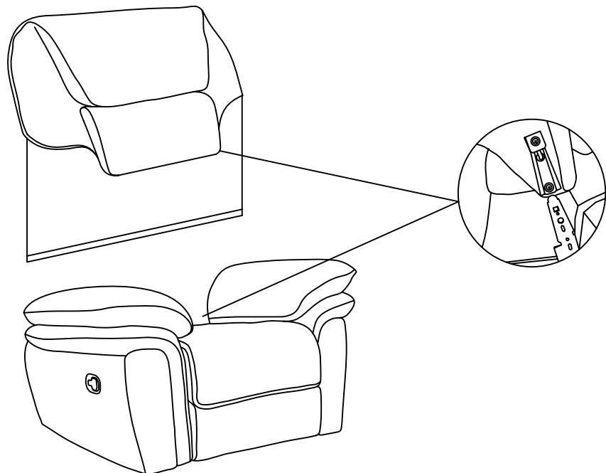
STEP 2 Pull on release lever to operate reclining mechanism
