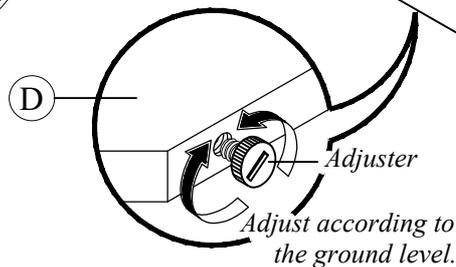
**NOTE : MUST TIGHTEN SCREWS PERIODICALLY WITH USE SCREW WILL BECOME LOOSE. CHECK TIGHTNESS OF ALL SCREW EVERY 6-8 WEEKS.**
