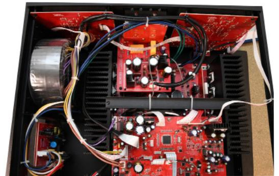
Advance work to stand out focuses on quality essential food linear, starting with the transformer 15 cm toric, tracking filtering by four capacitors 6800  $\mu$ F / 71 V, then multiple regulations also very well filtered for each circuit from A10.
