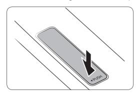
**1.** To unlock the adapter cover, press the cover to the left of the word PUSH as shown in the illustration.
