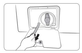
3. Put an empty, spacious container around the cover, and stretch the emergency drain tube to the container while holding the tube cap (A).
