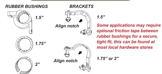
1) Determine the size of rollbar for your vehicle, install rubber bushings on rollbar 2) Insert and align notch of rubber bushings into the aluminum brackets 3) Apply supplied Loctite to allen bolt tips, then align the allen bolts and T-nuts into the T-channel, firmly tighten. Let dry for 20 minutes. Fully cures in 24 hours. 4) Recheck all allen bolts are tight, ensure T-nut's are properly seated in the T-channel correctly
