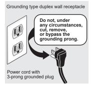
Use a dedicated grounding-type duplex electrical outlet for each unit (i.e. two duplex outlet receptacles, each on a dedicated electrical circuit) for a paired unit configuration
