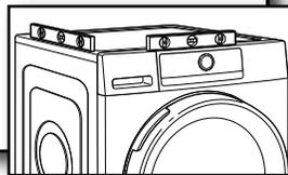
Remove cardboard from beneath washer. Place a level on top edges of washer, checking each side and front. If not level, tip washer and adjust feet up or down as shown in steps 15 and 16, repeating as necessary.
