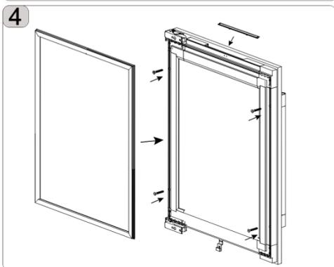
4. Use 4 long black screws to drive through the door from inside of the glass door into the wood door.
