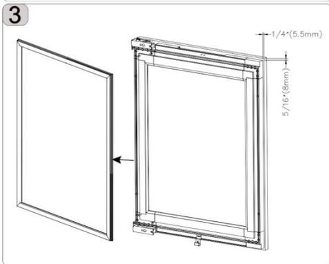
3. Remove the glass door seal, then measure adjust the wood door so that it is centered left to right with the glass door, approximately 1/4 inch (5.5 mm) above the glass door
