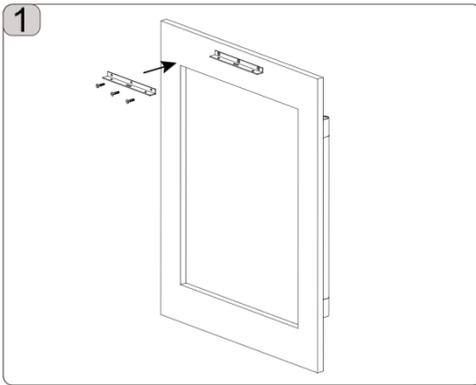
1. Fix the connecting plate to the corresponding hole in the wooden door.
