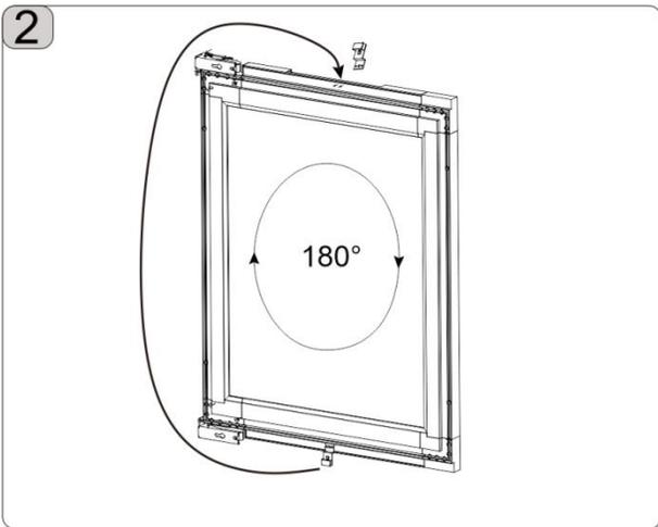
2. Remove the induction magnet unit from the bottom of the door and secure it to the other end of the door.
