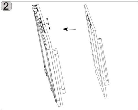
2. Hang the wooden door on the glass door, secure it with screws and adjust the bolts on the left and right sides to bring the wooden door to a satisfactory relative position to the glass door. Note that the bolt in the center is different from the specification of the two Sides.
