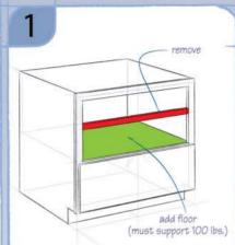
Remove top two drawers, drawer slides and stile. Add support surface. Must support 100 lbs.
