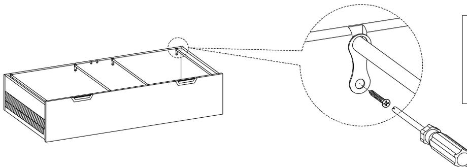
Remove the wood screws on the back panels of drawer box to remove the rod loops and file rods if necessary.
