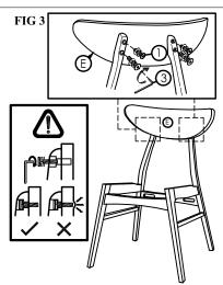
Step 3.1 Align bolt holes on Backrest (E) to bolt holes on both right and left Side Frame. Use JCBC Bolt with washer (1) and Allen Key (3) to fasten (E) into Left and Right Frame as shown on FIG 3.
