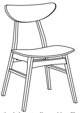
Step 6. Turn the chair to standing position. Check the chair for balance and tighten all the bolts to complete the assembly.
