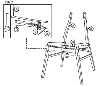
Step 2 Insert JCBC Bolt with washer (2) through the hole on Front Stretcher (C) and Back Stretcher (D) and tighten by using Allen Key (3) to screw into the hole on Left Side Frame (A) and Right Side Frame (B) as shown on FIG 2.
