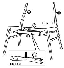
Step 1.1 Attach Front Stretcher (C) and Back Stretcher (D) via pre-installed wood dowel into the hole at Left Side Frame (A) and Right Side Frame (B) as shown on FIG 1.1.
