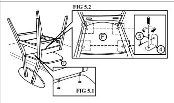
Step 5.1 Place the Seat Panel (F) upside down on a protective surface such as a covered table, Align the chair frame assembly as shown on FIG 5.1 and attach to (F) via wood dowel on Left Side Frame.
