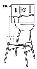
Step 4 Insert Wood Dowel (6) into the designated hole at Left Side Frame (A) as shown on FIG 4.
