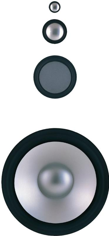
Each drive unit has been developed to operate as a piston within its intended frequency band, with two octaves between the upper roll-off and the first sign of break-up modes. Extensive use of aluminium in the diaphragms makes this possible. All voice coils are wound on polyimide formers to eliminate eddy-current losses, which are particularly serious at high frequencies.
