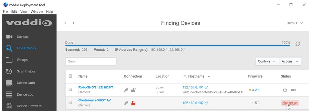
5. For each device that you need to work with, click the Not Set Up button and set the admin password on the device detail page that opens.
