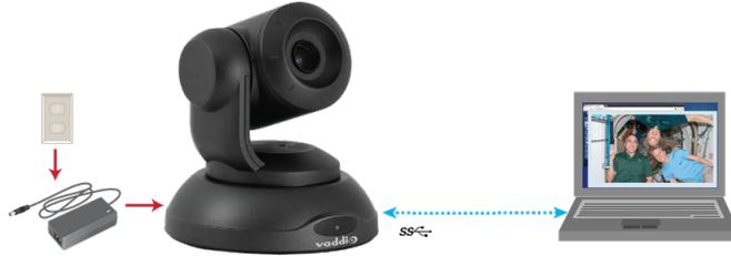
2. Connect power. The camera moves and the indicator light turns blue.
