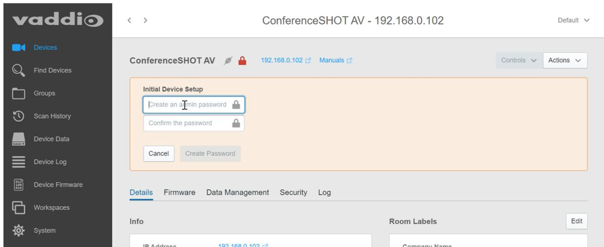
The device shows up as unlocked after you set the admin password. You can now access the administrative web interface to complete system administration and other configuration tasks. That's it. No complicated procedures for finding all the newly installed devices on your network. You can find and manage your whole Vaddio deployment from the Vaddio Deployment Tool.
