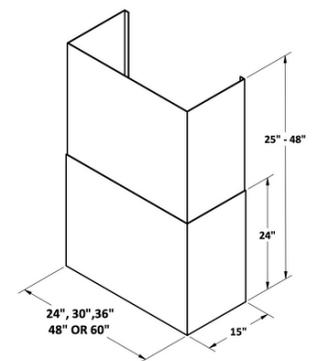
**DUCT COVERS:** MODEL #: PDC7236, PDC7242, PDC7248, PDC7260, PDC7272
