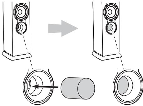
**CAUTION: Be careful not to insert the port plug so far into the port tube that it falls inside of the speaker.**
