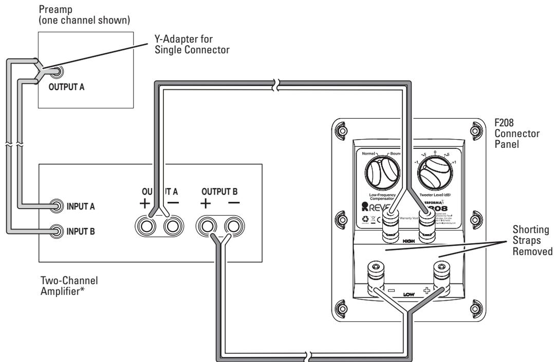
\*Amplifier for other loudspeaker must be identical
