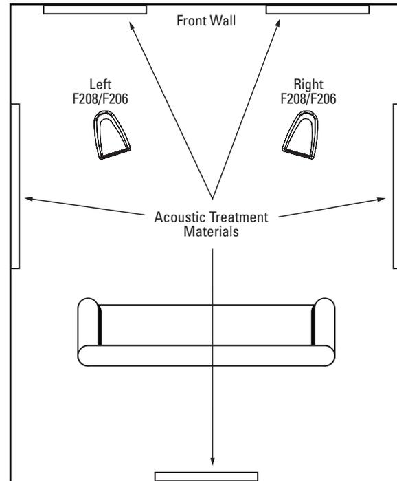
Because the listener's eyes and ears are on the same plane, the "mirror method" is an accurate determinant of critical reflection points. This method can be used to determine reflection points for side walls, rear walls, front walls, and even the ceiling. Applying acoustic treatment materials to the side walls is most important, followed by the ceiling, front wall and rear wall.
