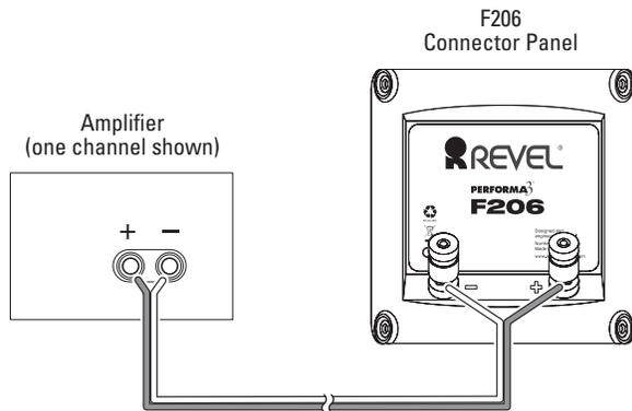
Connect both loudspeakers using the same method, using speaker cables of the same length for each speaker.
