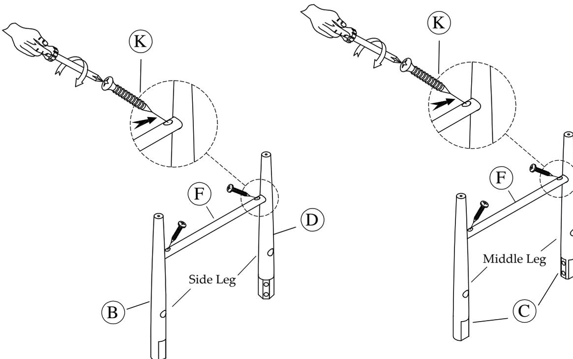
STEP 2: Do not fully tighten the bolts.
