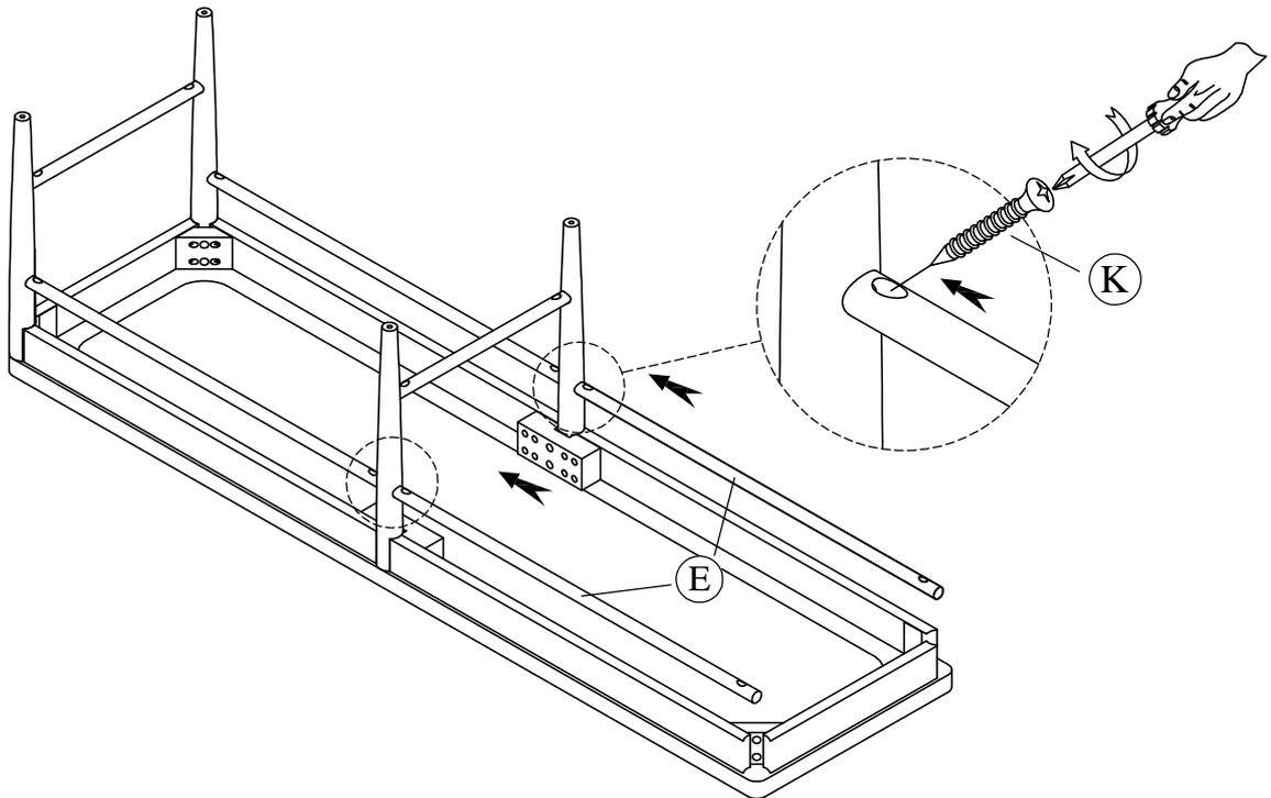
STEP 6: Using the Allen key and a Phillips head screw driver, tighten all bolts, then tighten all screws.
