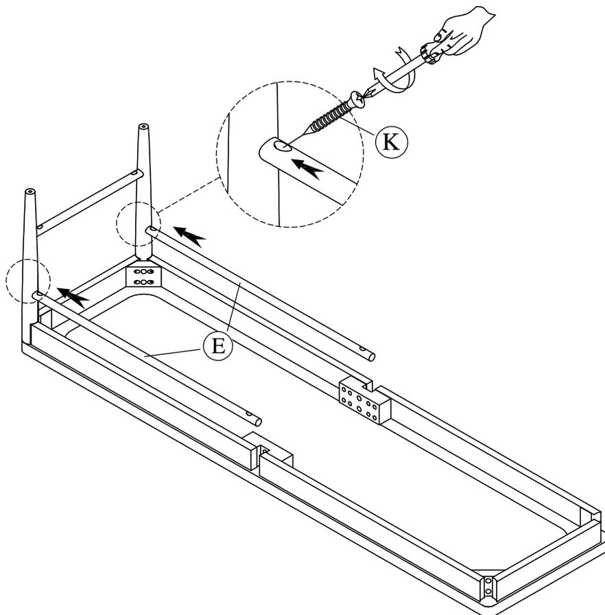
STEP 4: Do not fully tighten the bolts.
