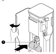
Open the right door and insert the combination tool 2, the crevice tool 3 and the cleaning brush **4** for storage.
