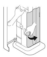
**3** Hold the product with one hand and take out the motor protection filter with the other hand
