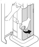
3 Press ▲ button **1** above the **PUSH** label with one hand. The dust bag is released.
