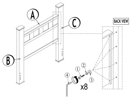
STEP 1: Assembly the Headboard Post L/R First attached the Headboard Post Left (B) and Headboard Post Right (C) to the Headboard (A) Using Allen Key (4) to tight Flat Washer (3), Spring Washer (2) and Allen Bolt (1).
