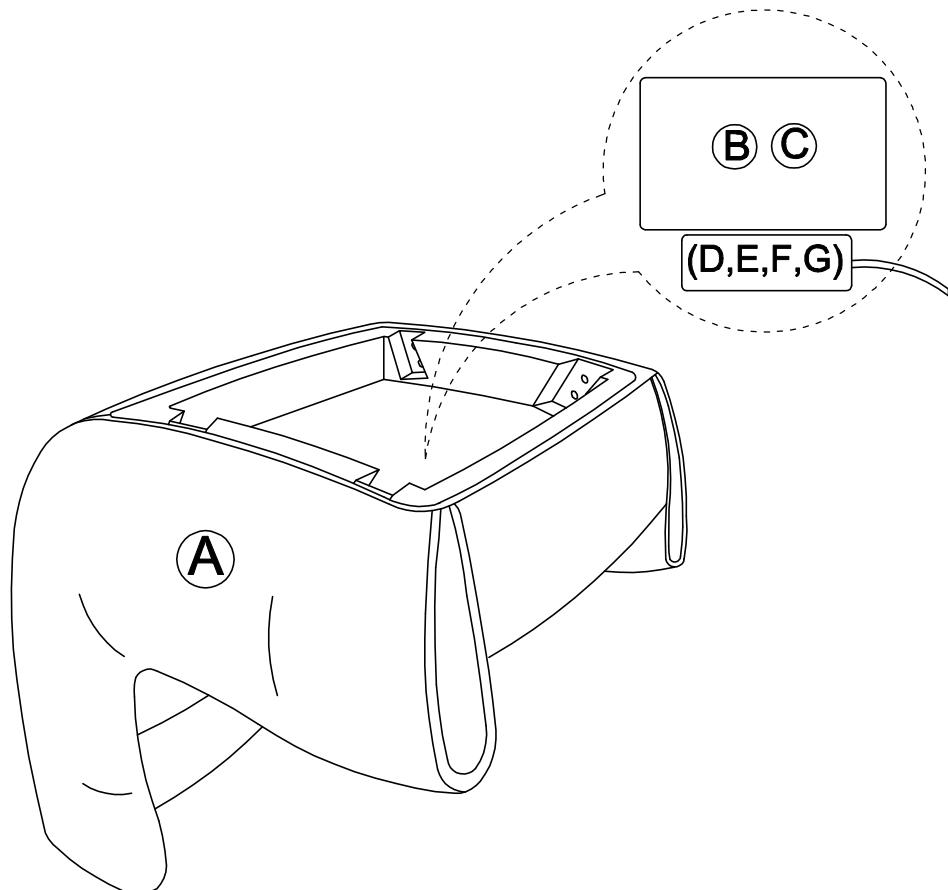
**STEP 2:** Insert Wooden Rear Leg(B) in to correct location.
