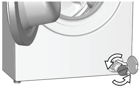
4. Clean any residues inside the filter as well as fibers, if any, around the pump impeller region.
