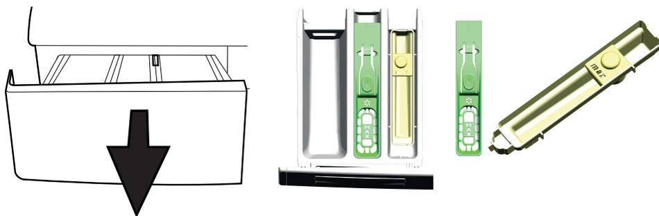
1. Press the dotted point on the siphon of the softener compartment and pull towards yourself until it is removed from the dispenser.
