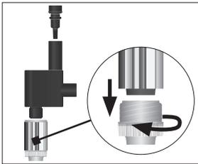
If insufficient foam is produced when the milk is frothed or milk sprays out of the fine foam frother, this may get dirty. If this happens, dismantle and rinse the fine foam frother.
