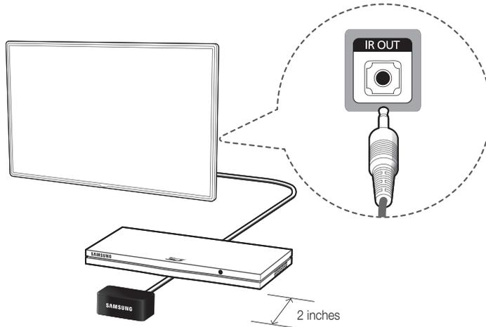
Keep a distance of 2 inches at least between the IR Extender and the external device, as the illustration shows. Face the IR Extender toward the external device's remote control signal receiver. Note that it should be no obstacle between IR Extender and external device. The presence of an obstacle will interfere with the transmission of the remote control signal.
