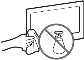
Do not spray water directly onto the product. Any liquid that goes into the product may cause a failure, fire, or electric shock.
