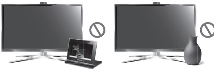
Do not block the sensor with any material. It can decrease picture brightness.
