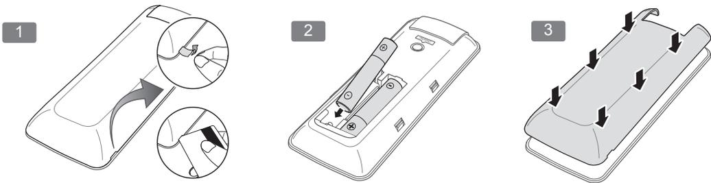
1. Slightly lift the battery cover by pulling the strap or using a plastic card (e.g. a credit card). Next, pull on the cover's notch with a fingernail to remove the cover completely.
