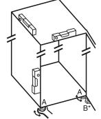
Then prop up the door: Screw out the adjustable foot on the bearing bracket (B) using the open-ended wrench SW10 until it comes into contact with the floor, then turn an additional 90°.
