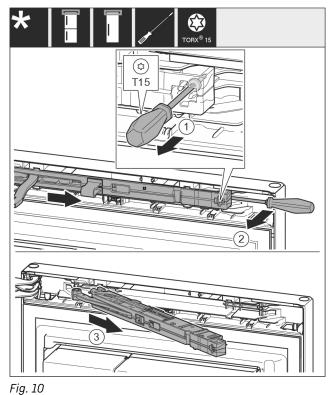
Loosen the soft stop unit screw with a T15 screwdriver approx. 14 mm (0.55 in). Fig. 10 (1)
