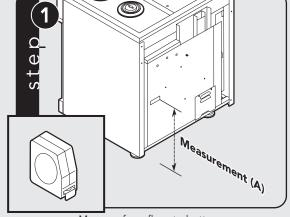
Measure from floor to bottom of the anti-tip opening located on the back of range. This will be measurement (A).
