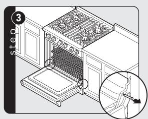
Remove pins from holes in hinges.
