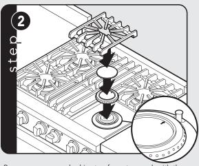
Burner caps are packed in styrofoam top pack with the grates. Place burner on top of range. Place burner grate on top of burner cap and grate support. **Note:** Arrow on burner cap must be pointing towards back of range.
