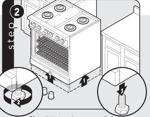
Note: It is strongly recommended that a pallet or lift jack be used rather than tilting.
