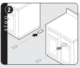
For uneven or sloped floors, level unit with metal shims only, as the adjustment required may exceed the thread available in the leg.
