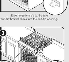
Check that unit is level side to side and front to back. The side trim must be 3/8" (0.95 cm) above countertop. If unit is not level repeat steps 5-7 of "Leveling/Adjustments/Alignment" section.
