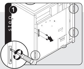
Unscrew four standoff brackets and remove.
