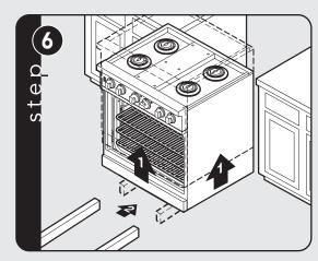
Lift unit and prop on wood blocks.
