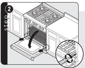
Open door completely. Reattach hinge trin
