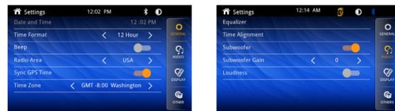
**Sync GPS Time:** Synchronizes the clock time with the GPS.
