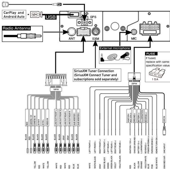
**Note:** When replacing a fuse, make sure to use the correct type and amperage. Using an incorrect fuse could cause damage. The unit uses (1) 15 amp ATC mini style fuse located on the power connector.
